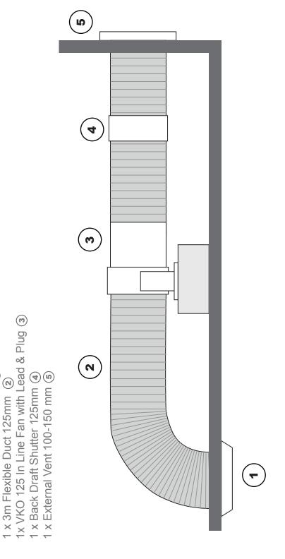
Internal cone vent 125 mm
